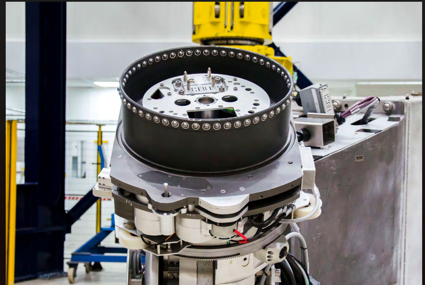
ARTICULATED BOOM WITH ODU-MAC® CONNECTORS AT EACH OF THE THREE ARTICULATED JOINTS – IMAGE COURTESY OF UKAEA RACE
