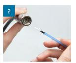
Insert cleaning stick into the connector and place it on the lens.
