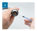
Insert cleaning stick into the receptacle and place it on the lens.
