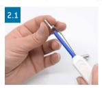
Put on the centering sleeve with the laser engraving "female".
