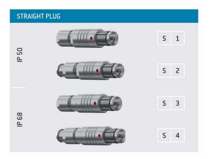
The Style S1/S2 and S3/S4 shown here are the two most commonly used straight plug housing styles. Housings styles S1 and S2 are IP 50 protected where styles S3 and S4 are IP68 protected in mated condition.
